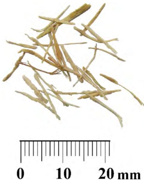
Fig. 1 – Processed sugarcane bagasse fibers.
