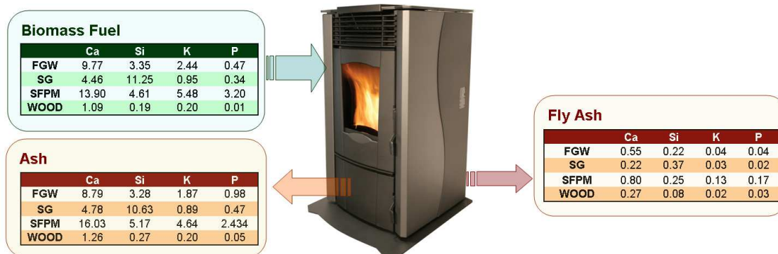
FIGURE 2: Mass balance of Ca, Si, K and P (values in g/kg biomass )
