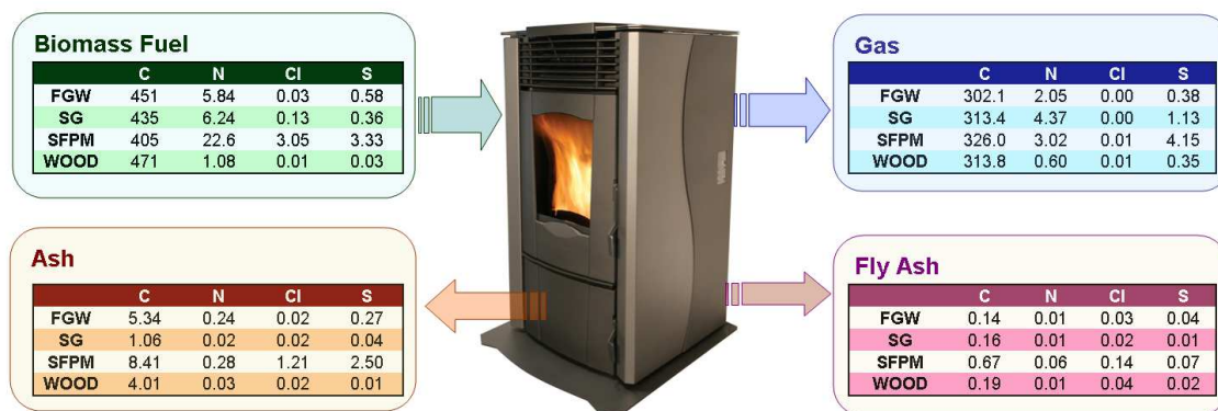
FIGURE 1: Mass balance of C, N, Cl and S (values in g/kg biomass )
