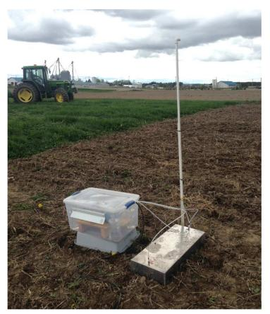
Figure 2. Photo of the chamber and sampling box in a no-till plot
