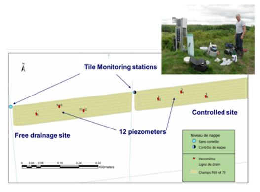
Figure 4-10. Location of the 12 observation wells and monitoring stations of the subsurface drain collectors.
